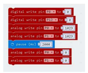
You can write a value from 0 to 1023 in the write\_analog statements. The higher your value, the quicker you move forwards. This would be a little under 80% speed.
