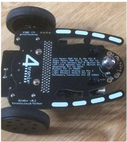
On the underside of the PCB there are two line sensors. These are far enough apart to follow the lines on the tracks I've used with other robot vehicles. There is also a helpful list of the pin connections which are,
