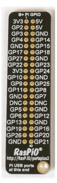
**GPIO** stands for **General Purpose Input Output.** Inputs are things like buttons, keyboards and sensors. Outputs are things like lights, buzzers and signals.
