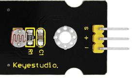
A black PCB module with a photocell sensor, a potentiometer, and a resistor (R1). It has three pins labeled +, -, S.                   |
