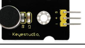
A black PCB module with a sound sensor, a potentiometer, and a resistor (R1). It has three pins labeled +, -, S.                       |
