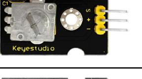
A black PCB module with a rotation sensor, a potentiometer, and a resistor (R1). It has three pins labeled +, -, S.                   |
