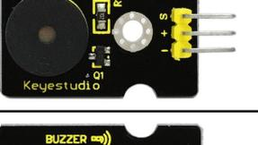
A black PCB module with a passive buzzer, a potentiometer, and a resistor (R1). It has three pins labeled +, -, S.                   |
