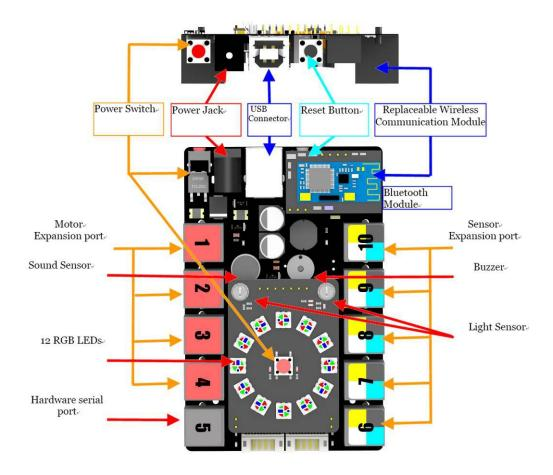
Based on Arduino Mega 2560, Me Auriga includes 10 easy-to-use RJ25 ports and 12 RGB LEDs. It integrates various sensors, such as gyro sensor, temperature sensor, light sensor and sound sensor.
