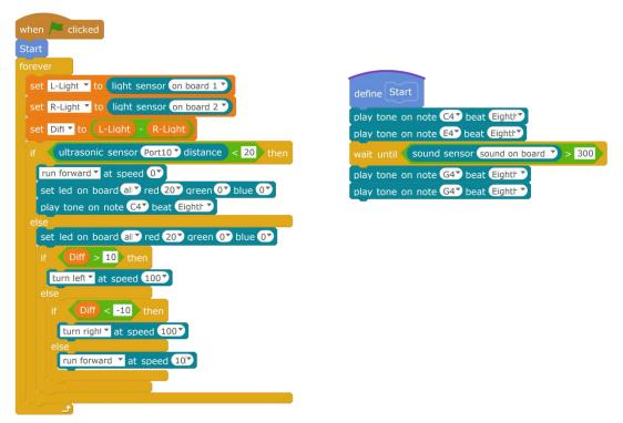
Have a try! Connect Ranger to the computer with USB cable and upload the program to Arduino to make Ranger start the program offline. Can it stop and make an alarm when it encounters obstacles?
