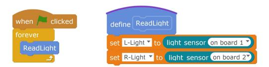
Please connect Ranger to the computer with USB cable to upgrade Ranger's firmware, and then click the green flag to start the program. The value of light sensor will keep bouncing. The increase or decrease in value of light sensor varies with the changing of ambient light. The brighter the environment is, the higher the value is, whereas the darker the environment is, the lower the value is.
