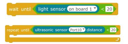
Please change the [Waiting] command in Target Task 1 program to [Repeat executing...until] command block, which executes other command blocks when the user is waiting for some conditions. Here we let the program to execute playing the tone command. You can also add LED light control. In principle, do not execute too many commands in repeated operations, in order not to affect the detection judgment of [Until...]. The program is as below:
