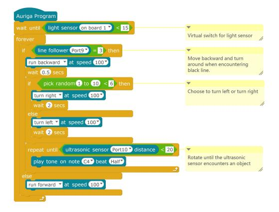
Have a try! Your robot will choose to turn left or turn right by itself, and is not restricted to one rotating direction any more. In this way, the robot seems to be given a life, which can choose its own rotating direction by itself. If you can make the most of the [Pick random 1 to 10] command, your robot will change more!
