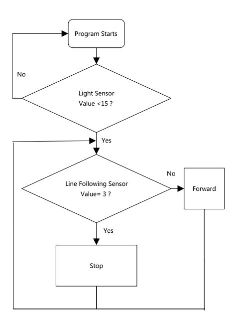
To avoid robot from starting motor and rushing forward at the beginning, we can use the [Wait until light sensor on board1<15] command and make a virtual switch. Let's control robot to start action.
