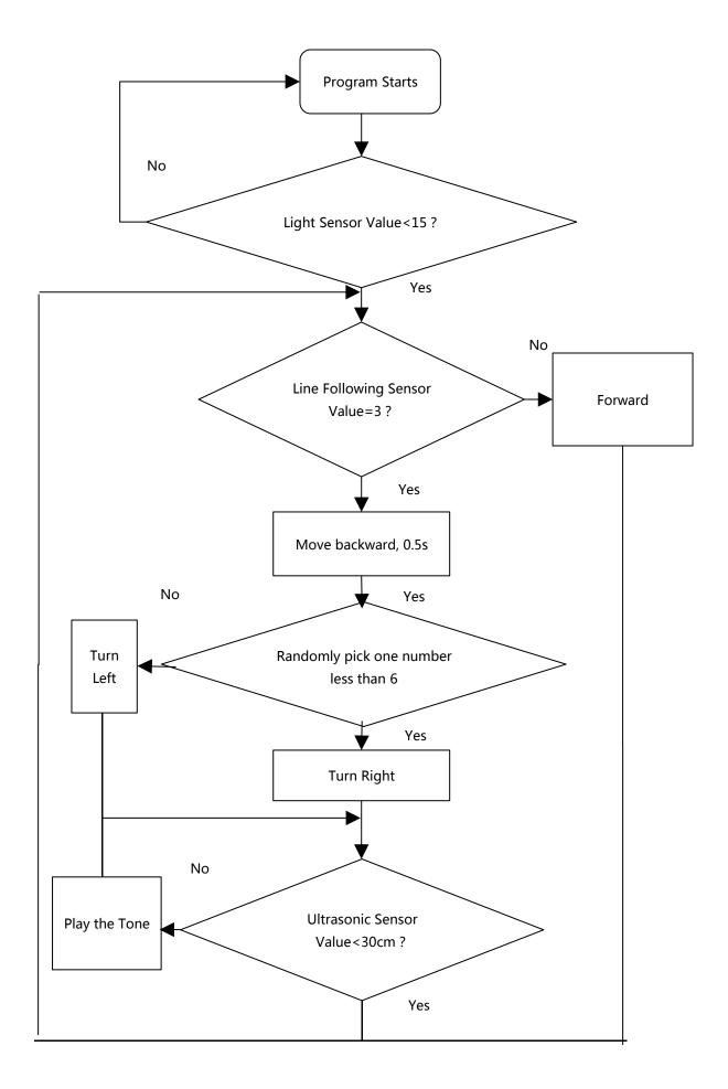
This program is used to replace the command of turning right only. The whole program is as below for reference:
