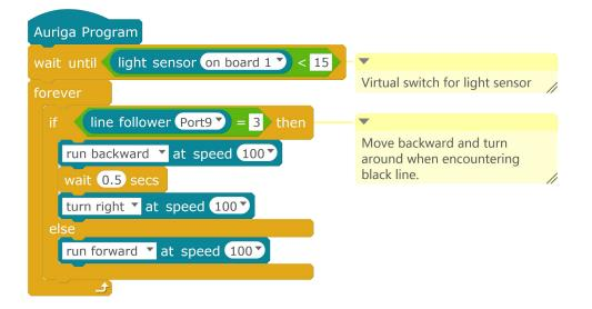
In the above program, mBlock Robots commands are used for moving and turning. You can also use the command of encoder motor to directly control the speed of motor, achieving turning effect.
