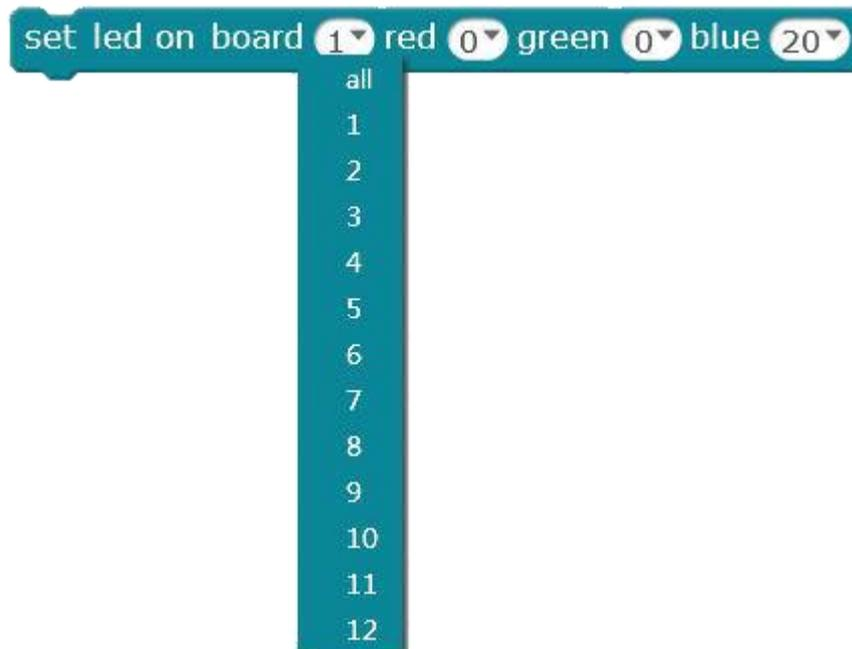
LED lights are arranged in a clockwise manner as follows: No.1 LED light is located near the middle of No. 7 and. 8 port on the left side of Me Auriga mainboard, followed by 2 to 12 LED lights. "All" means that all LEDs (12) are lit or turned off together.
