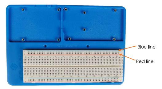
Then insert the T-Extension Board into the Breadboard, and insert the 40-pin GPIO Cable into the board.
